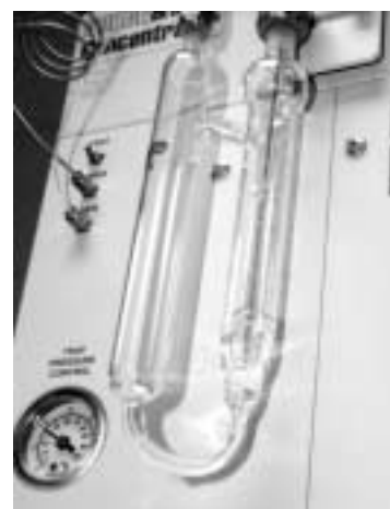
Sample purging in progress in a Tekmar 3100 concentrator.
