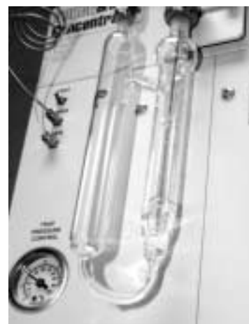
Purging a 5mL sample in a 25mL purge vessel, to reduce water transfer to the trap.
