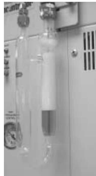
Wastewater samples commonly contain surfactants and other material that can contaminate the concentrator.
